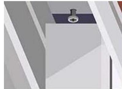
Supplemental locks or pins can also be installed at the top and/or bottom, and/or wooden dowels can be placed in the inside bottom track to prevent the door or window from opening.
